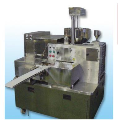
Firstly, put stuffing into the stuffing hopper, then put the prepared pastry on the transfer table by hand, after that the samosa machine automatically deposits the stuffing on the pastry, wraps / folds the stuffing through 3 steps, glues, finally delivers them onto the conveyer.
